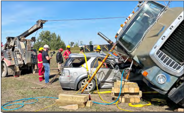
There were 12 students involved in the training days. Here students lift a water truck off a passenger vehicle using struts, airbags and hydraulic lifting tools.
